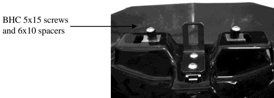
Before tightening completely, place the seat cover on the bike, center it (move the position of fasteners if necessary), remove it and tighten screws so as to block the fasteners location.
