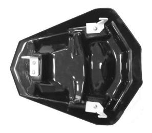
Before final tightening, offer the seat cowl up to bike & centre it, (by adjusting position of staples if necersary). Once happy remove seat cowl and final tighten all screws to lock the brackets into position.
