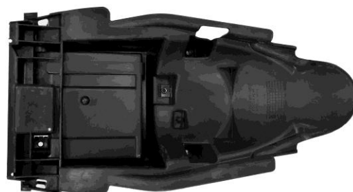
Original undertray after cutting
