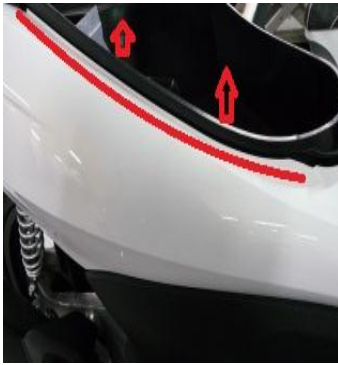
Pull up the bin so as to clear the edge at the red line level
