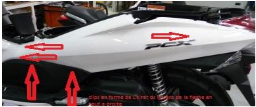
Clips' location : pull in the direction of the arrow at the right top to exit the fairing
