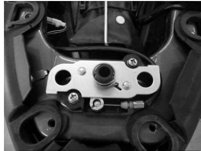
2° Position of the locking system of the saddle
