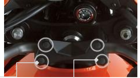
Photo 2 Screws to remove and replace
