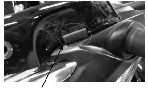
Position of pieces of rubber seal
