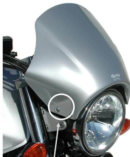
Nose screen fitting screw
