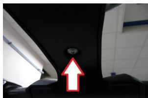
Phillips screw of the rear mudguard
