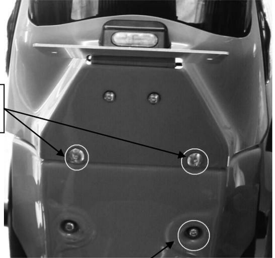
Fitting screw of the atmospheric captor
